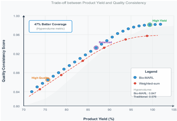
Figure 2. Pareto frontier visualization for multi-objective optimization
