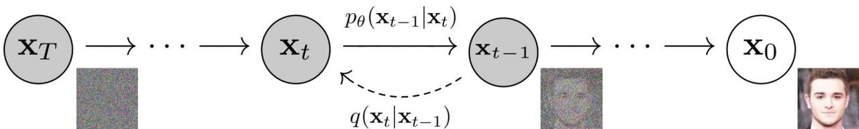
Figure 1 Illustration of a Denoising Diffusion Probabilistic Model (DDPM), showcasing the process of gradually removing noise from data to generate realistic synthetic outputs [11].
