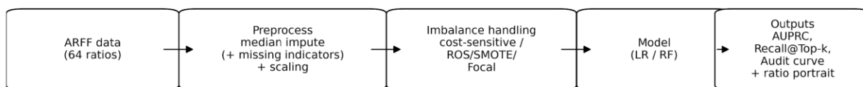
Figure 1. End-to-end workflow: preprocessing (including missing indicators), imbalance handling, model training, audit-oriented evaluation, and explainable ratio portrait.
