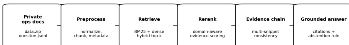
Figure 1. Evidence-grounded RAG pipeline evaluated in this study.
